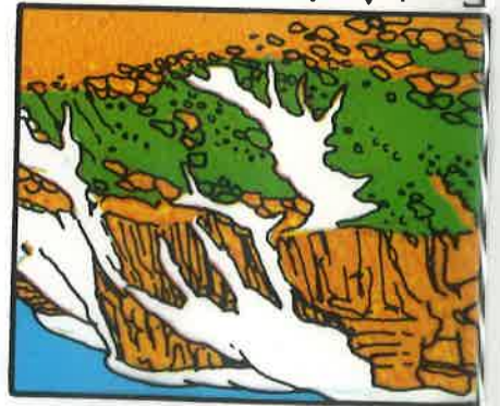
Frost Action repeated freezing and melting of water in pores of rock
